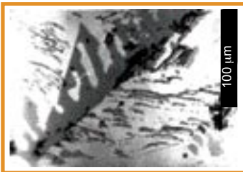
Current Conventional has dendritic growth resulting in less uniform microstructure
